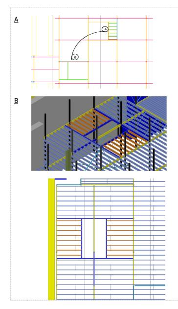
a) To move the existing stair from position A and fill in the opening with the required secondary steel and decking (as described above).
