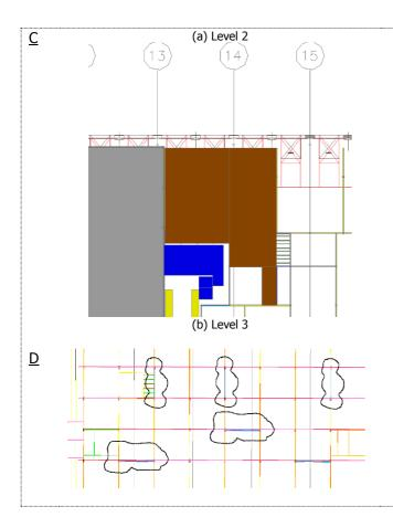
b) Level 3 - (brown) to supply and install required primary and secondary steelwork to the existing level 3 framing. To supply and install approximately 134m<sup>2</sup> decking and approximately 34m of free issue handrail & kicker to the edges. We have included for a Garment Hanging Stair between levels 3 to2. Handrail to the void edge is included.
